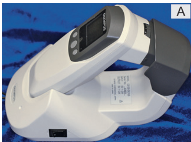
Fig 2 A dental spectrophotometer used in the present study. (A) Scheme of Crystaleye spectrophotometer. (B) Positioning on the black box. A custom holder was placed inside the box.
