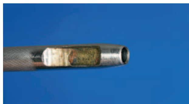
Fig 2 The punch to make the facial opening.
