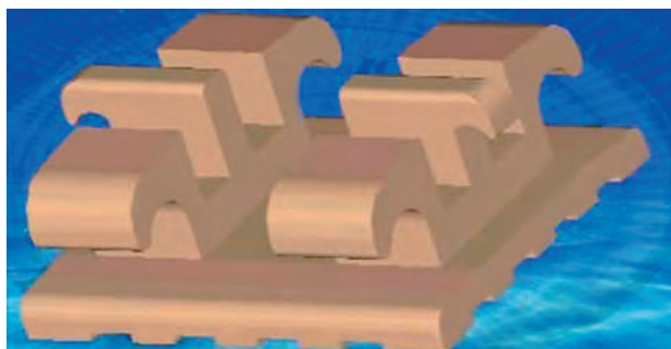
Fig 1 The Twin-slots bracket features two parallel 0.022" slots. The geometric form of the slots is rectangular with no built-in angulations at this preliminary stage.
